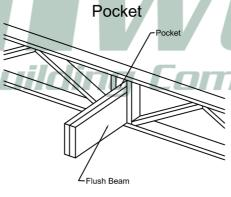
Flush beam to bear on all plies when a 2-Ply girder
