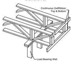
Truss Plating Not Shown For Clarity
