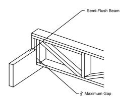
Truss Plating Not Shown For Clarity
