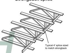
Connect a 48" splice member to strongback with 12 - 3" nails equally spaced along splice. Splice member shall be centered on splice joint and be of the same lumber size as the strongback.
